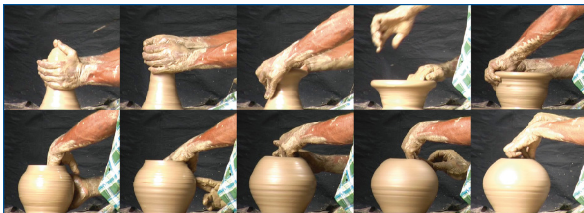
Figure 2: Examples of hand positions used during wheel-throwing. The images were extracted from a video recording of an Indian Multani potter throwing a 2.25 kg sphere (Gandon et al., 2013).
