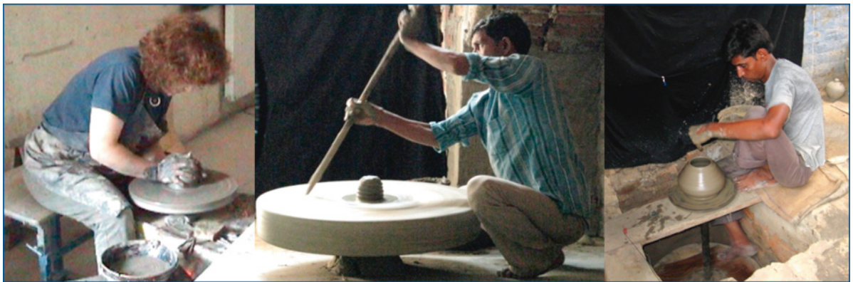
Figure 3: Wheels used in the three cultural settings. From left to right: the electrical (foot pedal operated) wheel used by the French potters, the high inertia stick-wheel used by the Prajapati potters, and the low-inertia kick-wheel used by the Multani potters.
